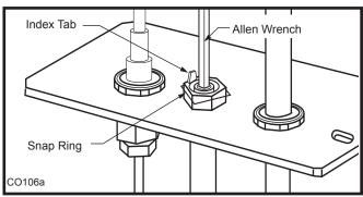
Fig. 10 Remove pilot orifice.
